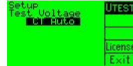
Test Voltage Selector Screen (CT Auto selected)
