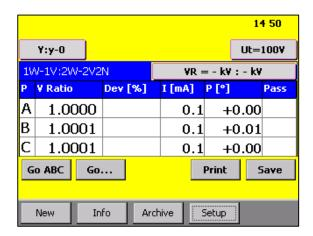
This is also the display you will find after switching on the instrument, if a measurement was finished before it was switched off.
