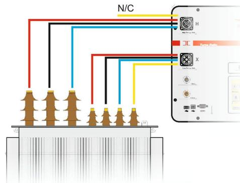
The colored leads are marked to indicate which transformer terminal it must be connected to for correct operation.
