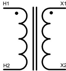
For example: The High Side Winding may contain 940 Turns: Low Side Winding 440 Turns.
