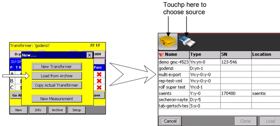
In the Archive screen, make your choice by touching on a transformer with your finger. Touch 'Load' to load it and append your measurement. Touch 'Clone' to create a new transformer, based on the one you have chosen.
